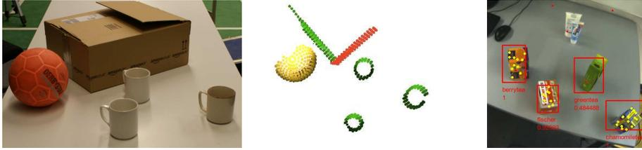
**Fig. 4.** Object Perception. Left: tabletop scene. Middle: points on extracted geometric shape primitives for the left scene (yellow sphere, green cylinder, red plane). Right: camera image (different scene) with rectangular object regions that are computed from object detections. The image also shows extracted SURF features (yellow dots) and recognized object class.
