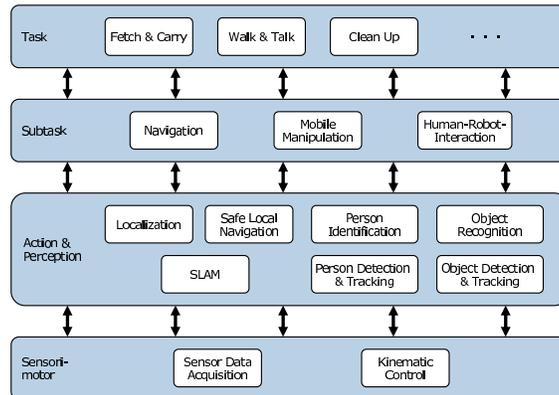
Fig. 5. Sketch of the control architecture.
