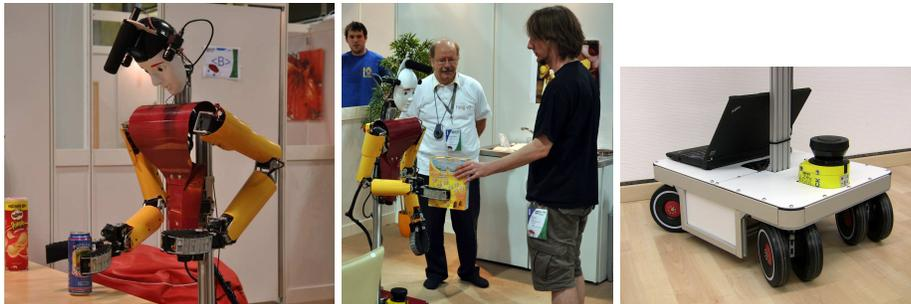
**Fig. 1.** Our robot Dynamaid with anthropomorphic arms and omnidirectional base.
